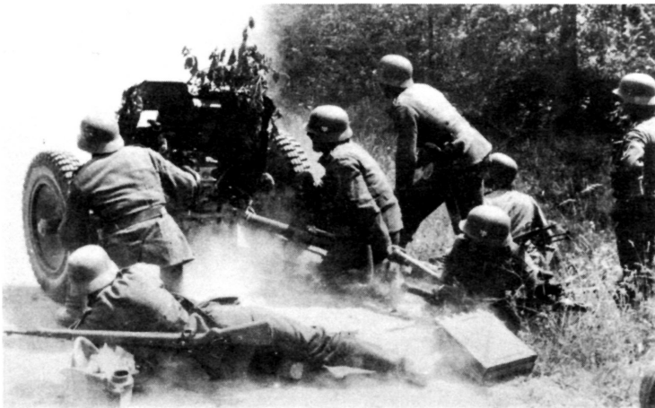
The 3.7cm Pak 35/36 was the best German antitank gun until 1941, when more powerful guns entered action. Its service life was extended during the war by the use of " Stielgranate 41 ," large hollow-charge stick shells with fins inserted in the muzzle. The caption on this photo says: " Panzerjaeger in defensive battle in Soviet Union." German Official Photo
