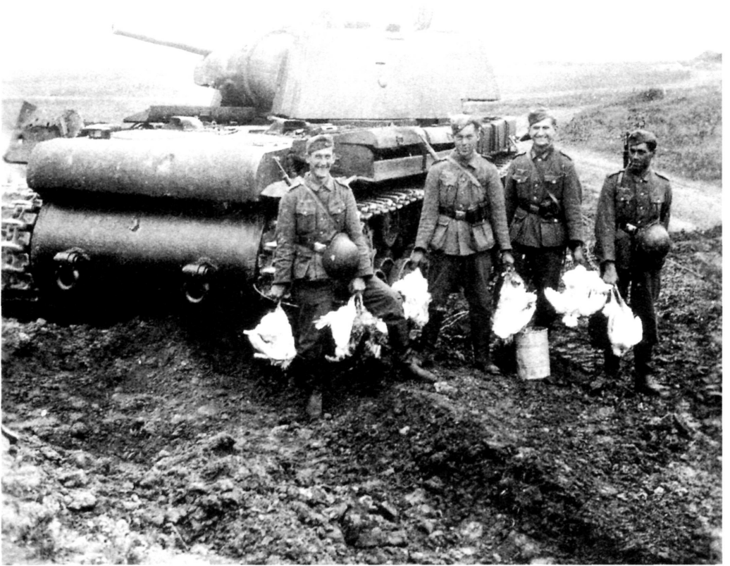
The spoils of war. German soldiers pose in front of a captured Soviet heavy tank with captured chickens. There will be a welcome change in the evening meal for their unit from the usual monotonous army rations. The tank, a 47.5 ton KV-I, had a 7.62cm gun as its main armament. German Soldier's Snapshot
