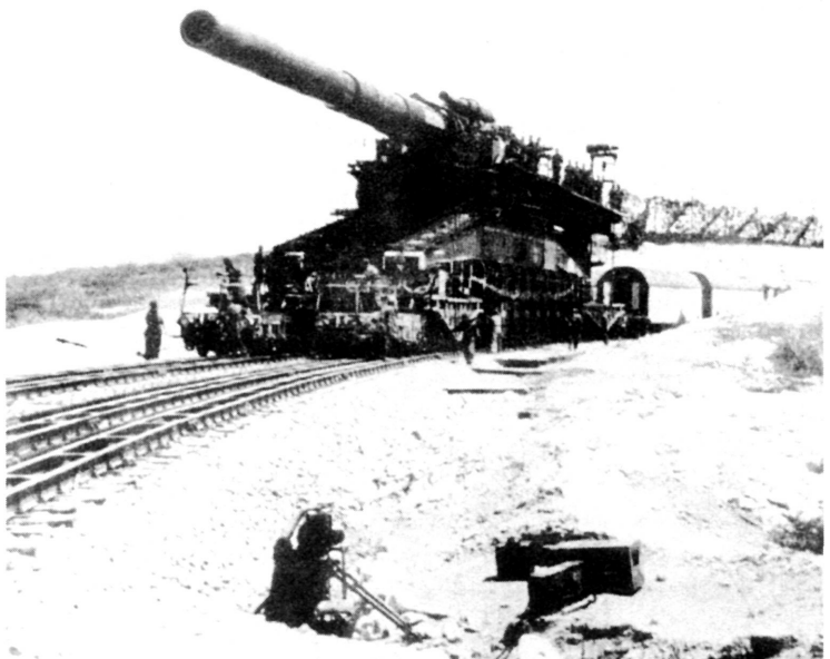
Dora on the curved, double-rail spur near Sevastopol in June 1942. The ammunition cars are behind the gun. U.S. Army Ordnance Museum
