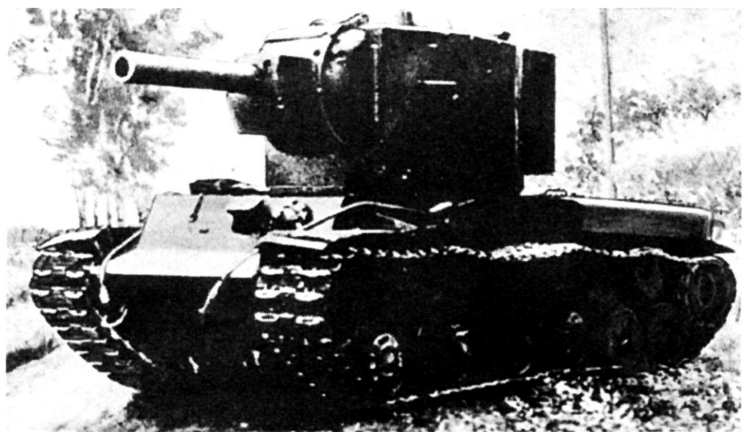
The Soviet KV-IIA was an artillery version of the KV tank with an impressive 15.2cm (152mm) M1938/40 L/20 howitzer in a high box turret. Built on the hull of the KV-I, it was found to be operationally ineffective during Barbarossa because of its weight of 57 tons, which made it slow, and a high silhouette of 13.7 feet compared to 8.75 feet for the KV-I. U.S. Army
