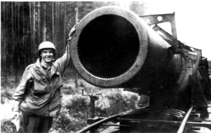
The muzzle of the barrel from the 80cm railway gun found scattered along the rail tracks near Grafenwoehr, Bavaria, by Col. F.B. Porter and the men of the U.S. Army 417th Field Artillery, in April 1945. U.S. Army Ordnance Museum
