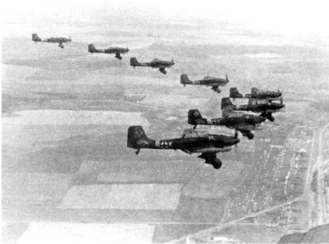
Junkers Ju 87D dive-bombers returning from a precision attack on targets during the summer of 1941. The Stuka, with a crew of two, was slow at 255 mph (410 km/h) and vulnerable because it lacked maneuverability, but it could carry up to 4,032 pounds (1,800 kg) of bombs. Smithsonian Photo
