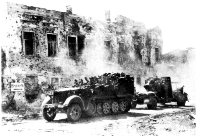
A German 8.8cm Flak 36 arrives in the battered port city of Kerch, pulled by its crew in a Sd.Kfz. 7 half-track prime mover. German Official Photo
