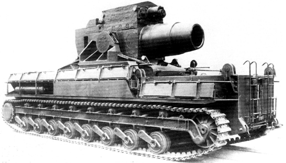
The left rear view of Karl howitzer No. 1 "Adam." The huge self-propelled gun, called a Moerser by the Germans, was designed to fire to the rear. The special concrete-piercing shell weighed 4,839 pounds (2,195 kg) and contained 617 pounds (280 kg) of high explosive. U.S. Army Ordnance Museum
