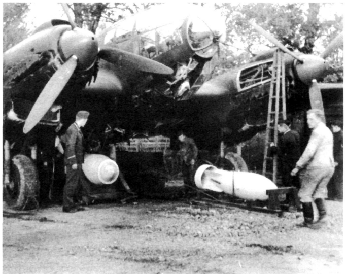
A ground crew prepares to load an SD 1700 bomb (left), about 3,750 pounds (1,703 kg), into the bomb bay of a Heinkel He 111H bomber. Note the Kopfring (head ring) to prevent excessive penetration. The bomb at right appears to be an SD 500 of 1,179 pounds (535 kg). Smithsonian Photo
