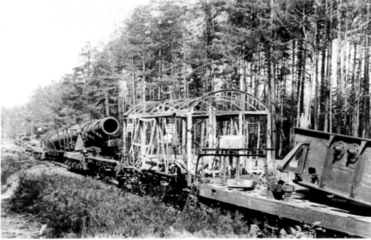
Dora's demise. The 80cm forward-barrel section ( Seelenrohr ), with the wreckage of an ammunition railcar in the foreground. This gun was destroyed by the Germans in April 1945 and parts from fourteen railcars were along some fifty miles of railway track near Grafenwoehr, Auerbach, and Weiden in Bavaria, northeast of Nuremberg. U.S. Army Ordnance Museum
