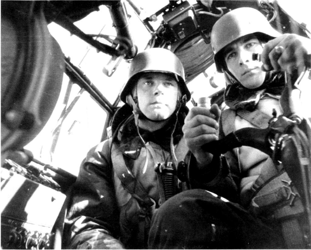
The pilot (right) and copilot-bombardier, in the cockpit of this Junkers Ju 88, are wearing standard Wehrmacht M35 steel helmets over their flying helmets as protection against enemy flak. A 7.9mm MG 15, on a flexible mount firing forward, is at the upper left. National Archives, Luftwaffe Collection
