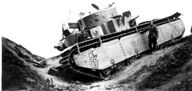
German infantry inspect a captured Soviet T-35B 45-ton heavy tank, knocked out during the breakthrough at Perekop. This obsolete tank was armed with one 7.62cm gun, two 4.5cm guns, and six 7.62mm machine guns. Author's Collection
