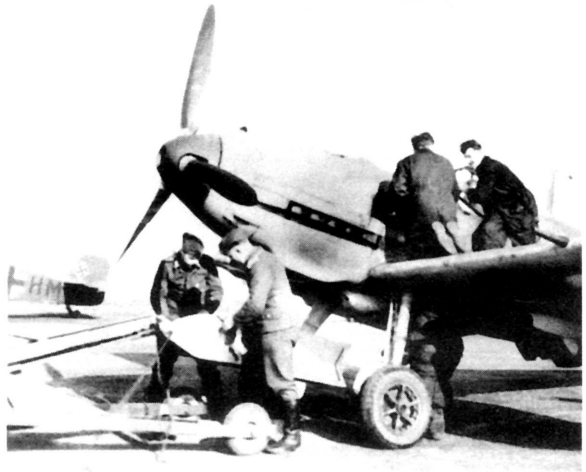
A ground crew with a special lift loads an SC 250 high-explosive general-purpose bomb, weighing 548 pounds (248 kg), under a Messerschmitt Bf 109E fighter-bomber. The Luftwaffe provided outstanding close air support to the German ground forces during the first months of Barbarossa. From Dr. Heinz Orlovius, Fliegen und Siegen (Munich, ca. 1942)
