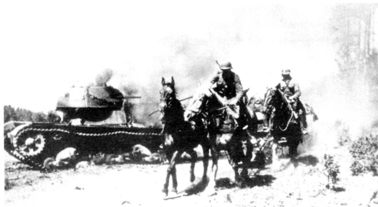
Barbarossa was a war of movement until the snow and bitter cold of the Russian winter froze virtually everything in its tracks. Here a German Army supply wagon, loaded with ammunition, gallops past a burning Soviet T-26S light tank. The turret and 4.5cm gun are aiming to the rear. From 5th Infantry Division, Mit uns im Osten (Stuttgart, 1942)
