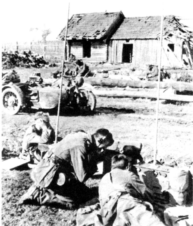
The Wehrmacht enjoyed the advantage of superior communications. A company command post receives instructions from battalion headquarters using the Tornister Funkgeraet b1 (Pack Radio Type b1), a transmitter/receiver with a separate case for battery and accessories. This radio, also used by the artillery, had a voice range of 10 miles and a C.W. range of 25 miles (16 and 40 km). Note BMW heavy motorcycle and sidecar, which has seen plenty of use. From Mit uns im Osten, op. cit.
