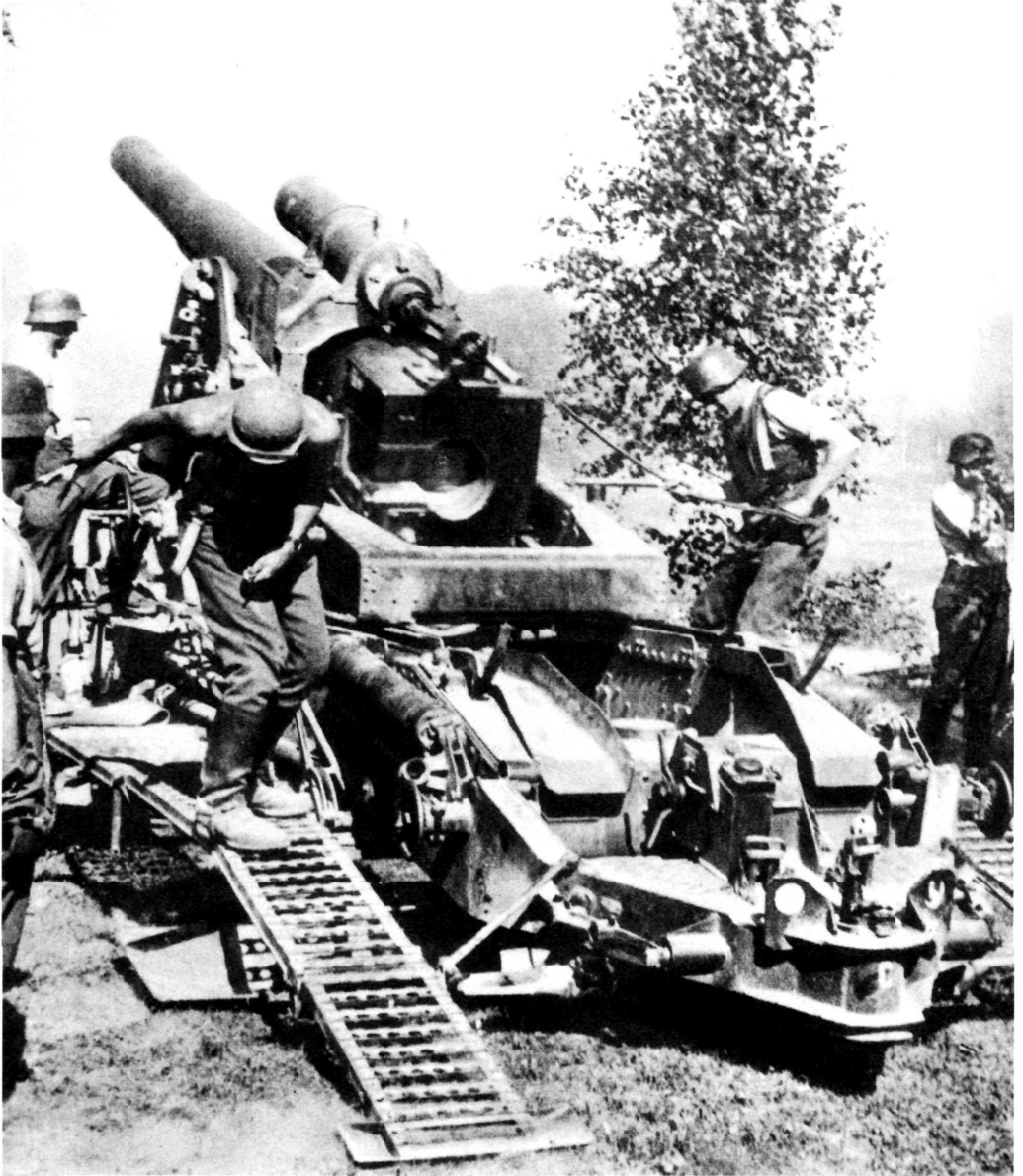
A German 21cm Moerser 18 at the moment of firing. This howitzer fired a wide range of ammunition and used a carriage similar to the 17cm K18. Maximum range with the standard high-explosive shell weighing 249.17 pounds (113 kg), with charge No. 6, was 18,290 yards (16,725 meters). From Infanterie im Osten , op. cit.
