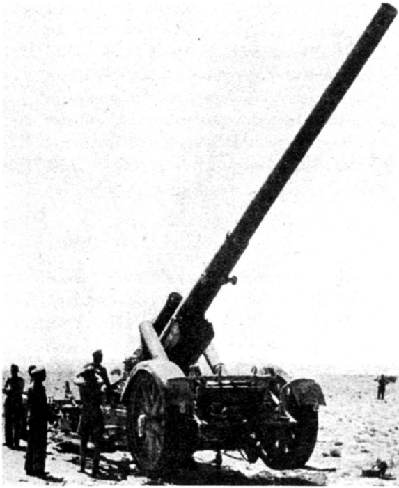
German 17cm Kanone in Mrs. Laf., a 170mm (6.7-inch) cannon on the 210cm Moerser 18 howitzer carriage, proved to be the best German heavy gun. Its 149.8 pound (68 kg) high-explosive shell had a maximum range of 30,621 yards (28,000 meters). The AP shell weighed 156.4 pounds (71 kg). From German Weapons Illustrated, op. cit.
