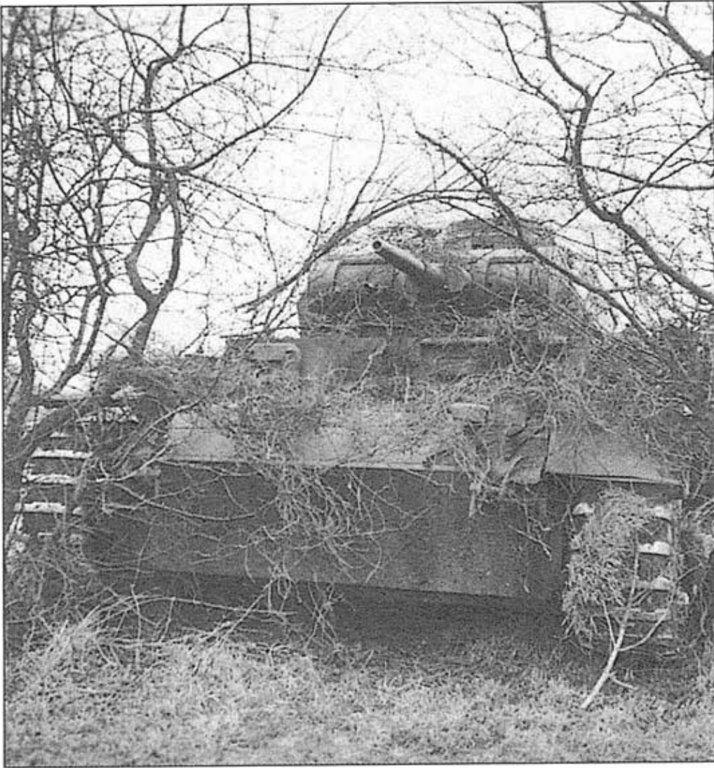
Left: A Panzerkampfwagen (Pz Kpfw) III, photographed in combat conditions. Armed with a 37mm or (as shown) a 50mm main gun and two 7.92mm machine guns, the Pz Kpfw III was the first German tank to go into mass production, entering service just prior to the invasion of Poland in September 1939.
