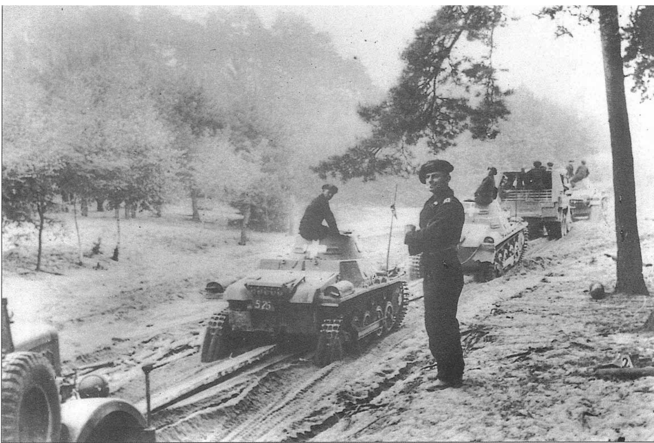
Above: A formation of Pz Kpfw I Ausf B light tanks of the 1st Panzer Division move forward through the dust of western Poland, early September 1939. The white crosses on the tanks are recognition symbols used just for the Polish campaign; they would soon be replaced by the more familiar black crosses lined with white (they made good aiming marks for anti-tank gunners!).
