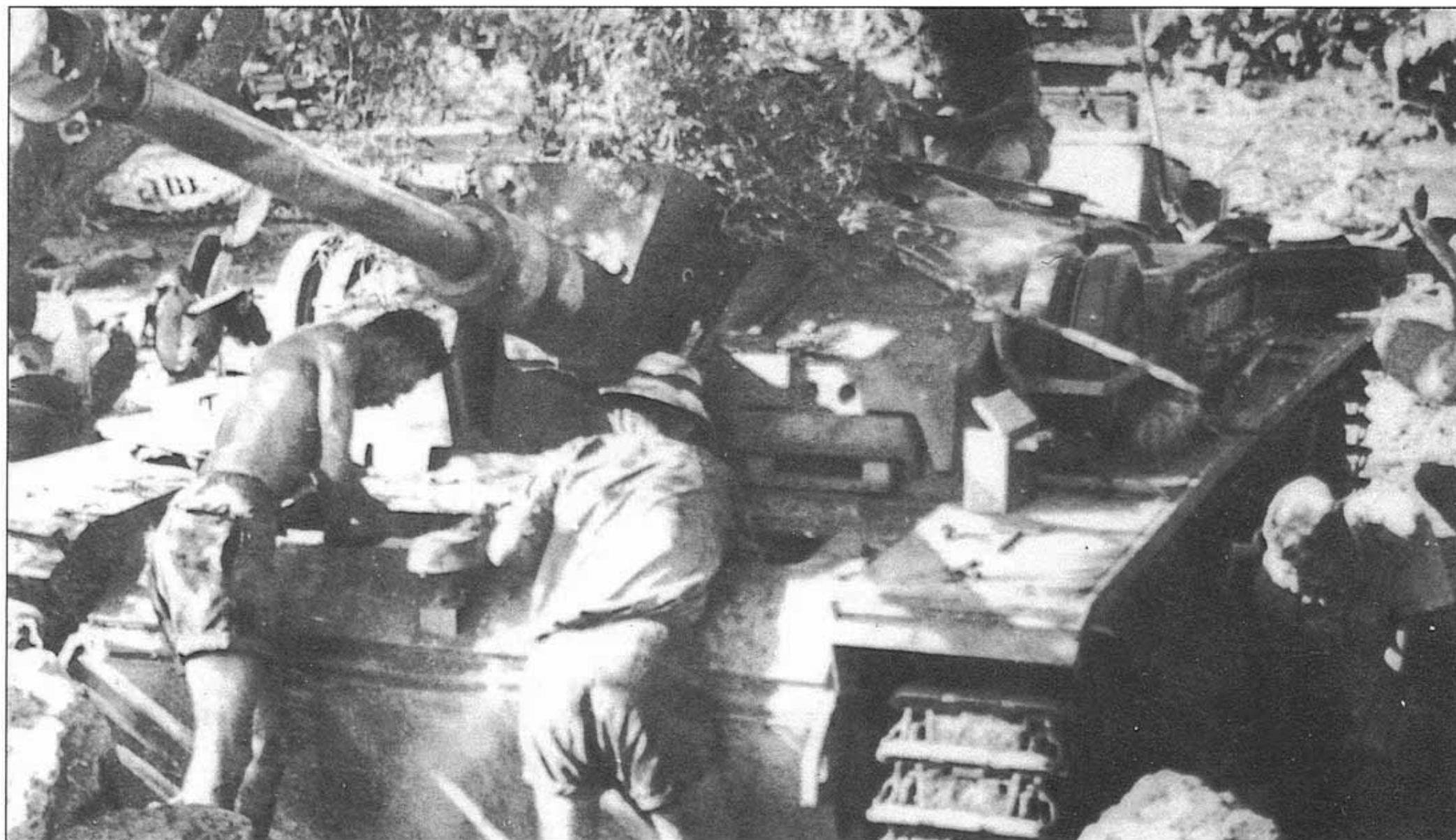
Above: Mechanics work on a Sturmgeschütz (StuG) III assault gun, taking advantage of the shade offered by a grove of trees in southern Greece, 1941. The StuG III was based on the Pz Kpfw III chassis, with a long-barrelled 75mm gun and 3in (80mm) of armour protection, and was used for infantry support.
