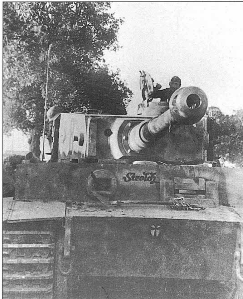
Left: A Pz Kpfw VI Ausf H Tiger I of the 508th Heavy Tank Battalion is photographed en route to Aprilia, Italy, 1944. The Tiger I was a very formidable fighting vehicle: with an 88mm KwK 36 gun in the turret and protected by up to 4.3in (110mm) of plate, it was superior to Allied tanks in both armament and armour.
