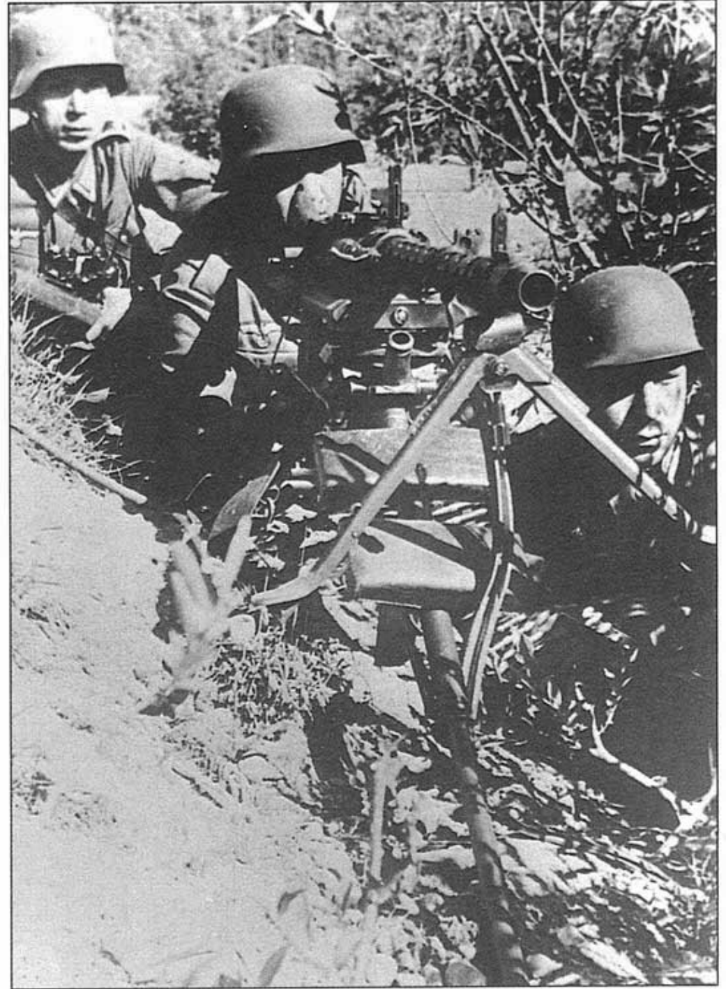
Above: The business-end of a 7.92mm schwere Maschinengewehr 34 heavy machine gun, well emplaced in a sheltered position in Russia, 1942. Mounted on a special Lafette 34 tripod, the weapon is configured for sustained long-range firing in support of infantry attacks.
