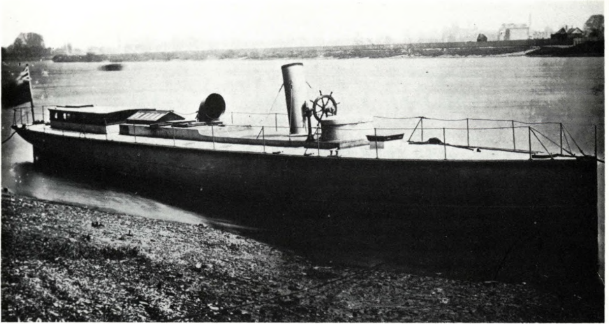
HMS Lightning in 1877, showing the amazingly exposed steering position
