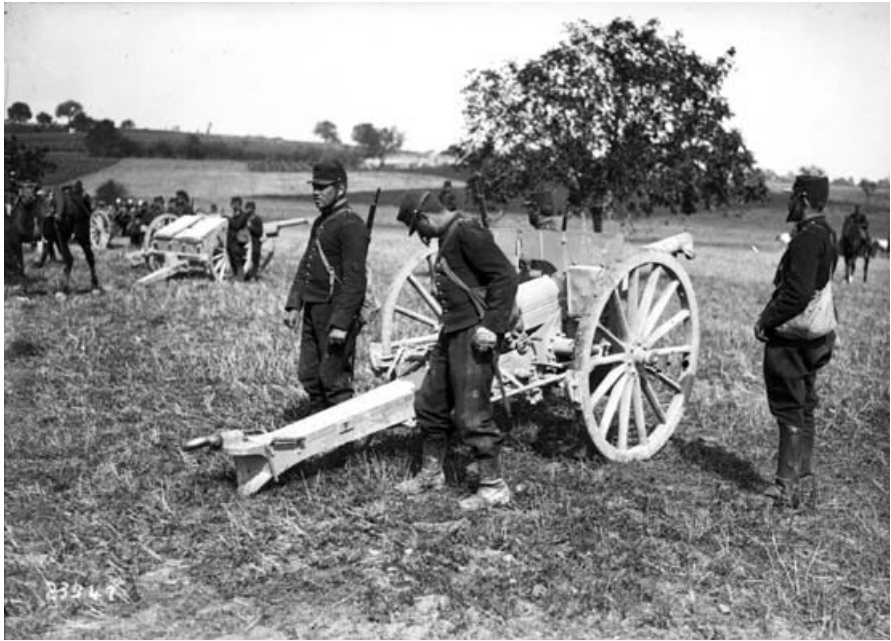
A French soixante-quinze Field Gun during the 1912 Manoeuvres. A formidable weapon in open country and a major factor in the French victory. (Bibliothèque Nationale de France)
