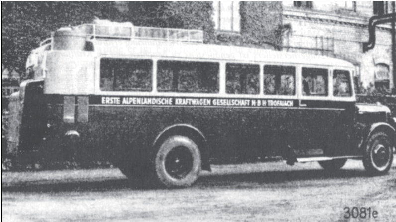
Illustration 1: A typical gaswagen which had originally been a conventional bus but which was subsequently retro-fitted with a gas-generator and a Saurer engine. 81
