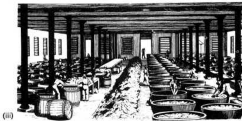
Figure 32. Soda manufacture using Leblanc's process: (i) shows the furnace in which the reaction takes place; (ii) shows the big vats in which the soda was dissolved out; (iii) shows the preparation of soda for the glass industry.
