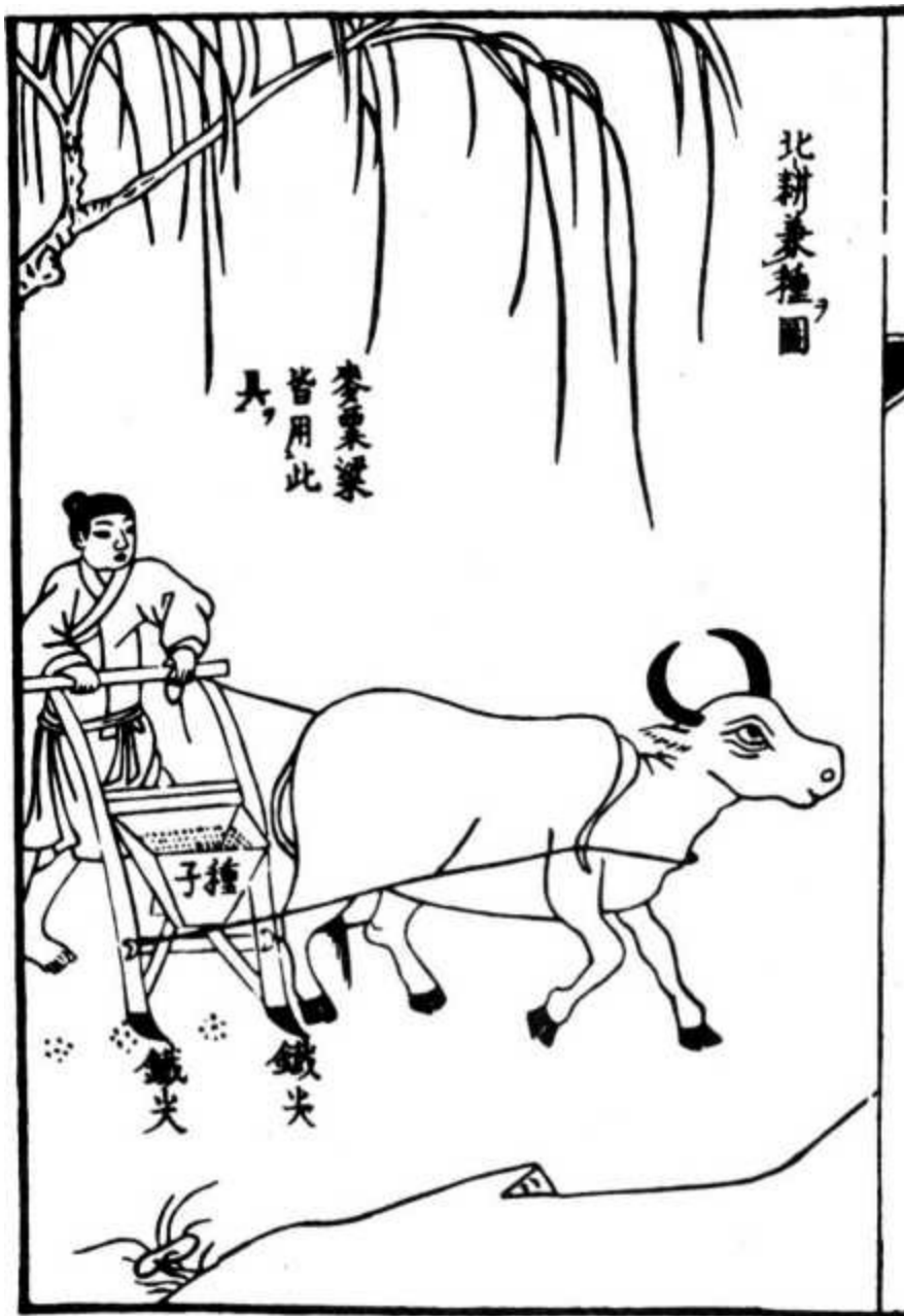
Figure 41. Chinese seed-drill used for sowing cereals, from the Thien Kung Khai Wu (Exploitation of the Works of Nature), 1637.
