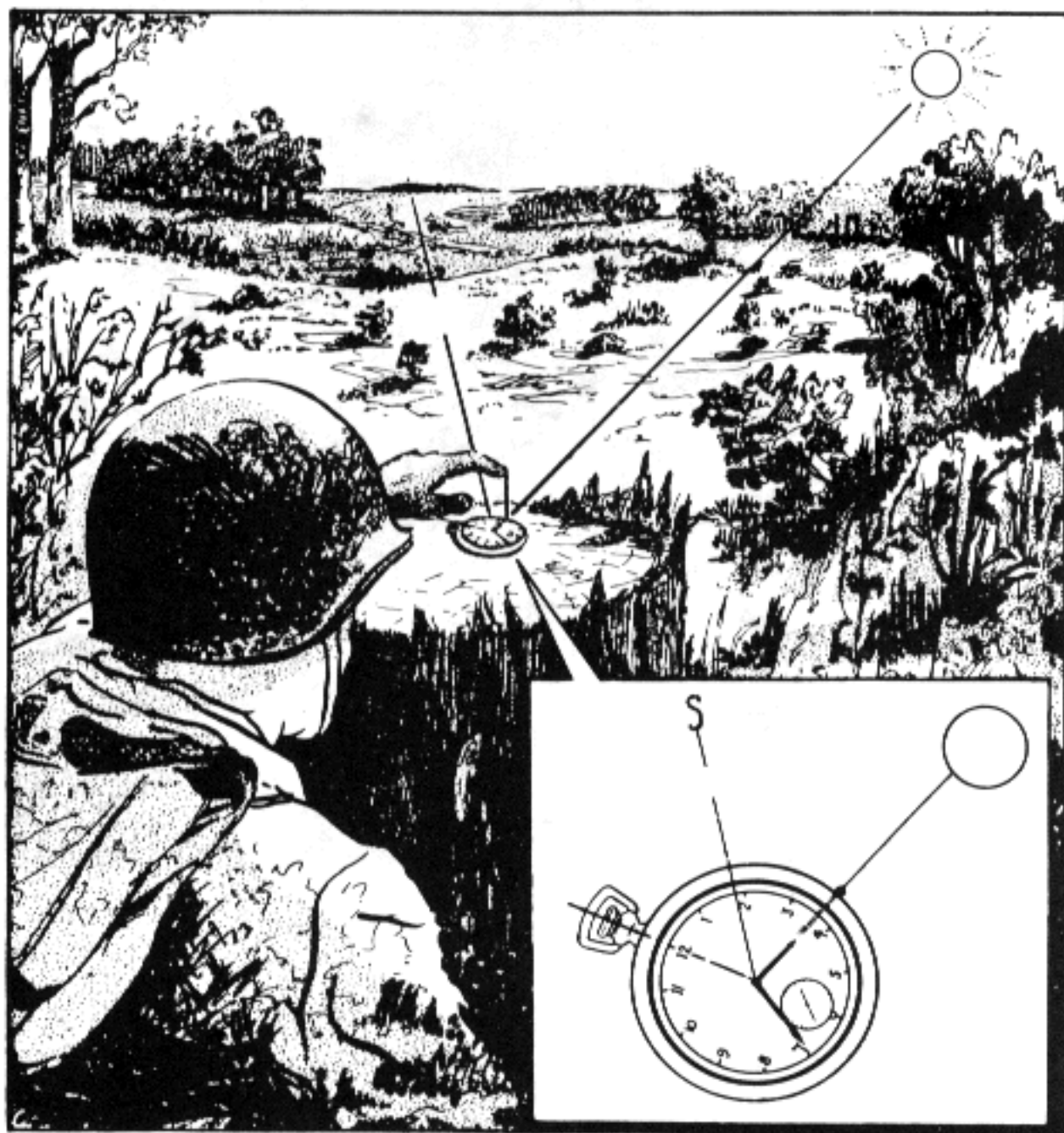
Figure 9. Sun and watch method of determining direction.
