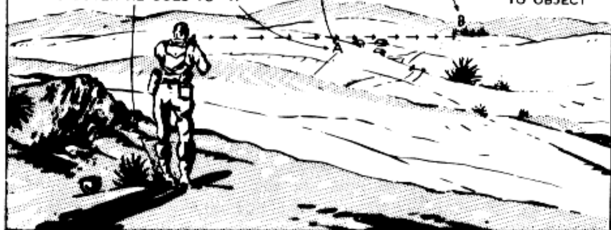
Figure 37. Method of obtaining azimuth, and marching by means of a compass.
