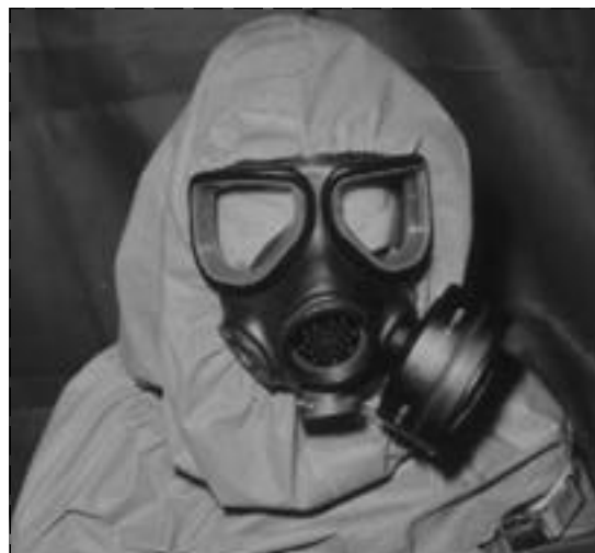
Fig. 16-7. The M40 Chemical-Biological Field Mask. Reprinted from Brletich NR, Tracy MF, Dashiell TR. Worldwide NBC Mask Handbook . Edgewood, Md: Chemical Warfare/Chemical and Biological Defense Information Center; September 1992: 385.
