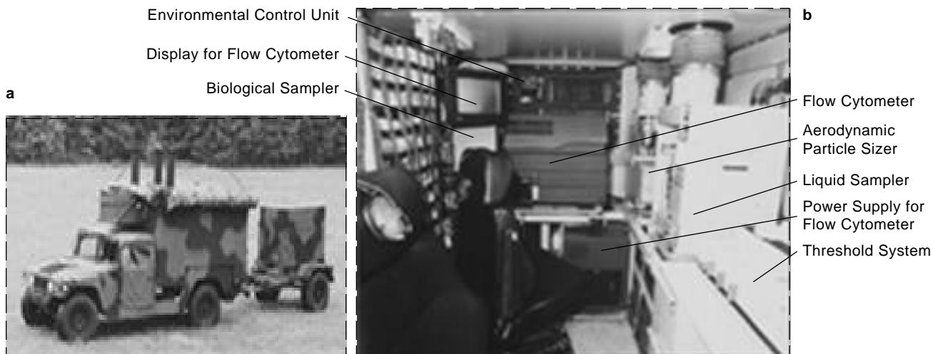
Fig. 16-32. (a) The XM31 Biological Integrated Detection System (BIDS) in its present configuration. Electric power is provided by a towed 15-kW tactical quiet generator. An additional high-mobility, multipurpose, wheeled vehicle (HMMWV) is used as a support vehicle for the crew of four, two of whom are required to operate the equipment that comprises the biological detection suite. The stovepipe-like structures perform the aerosol-sampling function. (b) Interior view of the biological detection suite. Photographs: Courtesy of Visual Information Division, US Army Chemical and Biological Defense Command, Aberdeen Proving Ground, Md.
