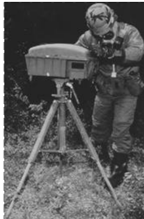
Fig. 16-30. Field use of the M21 Remote Sensing Chemical Agent Alarm (RSCAAL). Reprinted from Brletich NR, Waters MJ, Bowen GW, Tracy MF. Worldwide Chemical Detection Equipment Handbook . Edgewood, Md: Chemical Warfare/Chemical and Biological Defense Information Analysis Center; October 1995: 425. Photograph: Courtesy of Brunswick Corporation (now Intellitec), DeLand, Fla.
