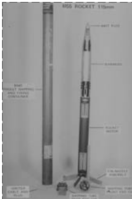
Fig. 2-52. The M55 115-mm rocket could hold the nerve agents VX or sarin. The problem was the aluminum warhead, which began leaking soon after production. Photograph: Chemical and Biological Defense Command Historical Research and Response Team, Aberdeen Proving Ground, Md.
