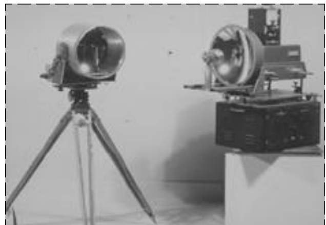
Fig. 2-48. A prototype long-path infrared (LOPAIR) alarm, the E33 Area Scanning Alarm consisted of an infrared source, optical reflector, optical collecting system, grating monochromator, and associated electronics. Photograph: Chemical and Biological Defense Command Historical Research and Response Team, Aberdeen Proving Ground, Md.
