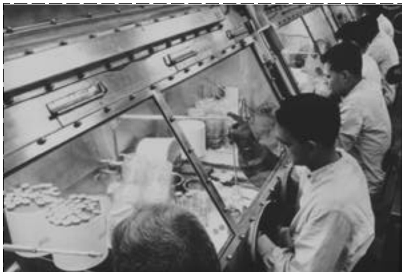
Fig. 19-2. Technicians in Class III hood lines are seen working with preparations of biological agents at Fort Detrick, Frederick, Maryland, circa 1968, when the United States had an offensive biological warfare program. The completely enclosed hood lines provide total containment of hazardous organisms. Hoods were maintained at a pressure negative to ambient by constantly drawing air out through high-efficiency particulate air (HEPA) filters. Workers wore heavy rubber gloves to access material inside the hoods. Photograph: Public Affairs Office, Fort Detrick, Frederick, Md.
