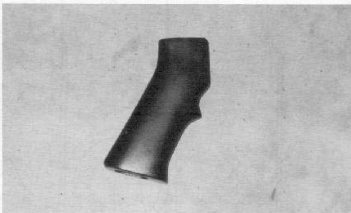
Grip was made of walnut, painted black simply because I didn't have a plastic military-surplus grip on hand.
