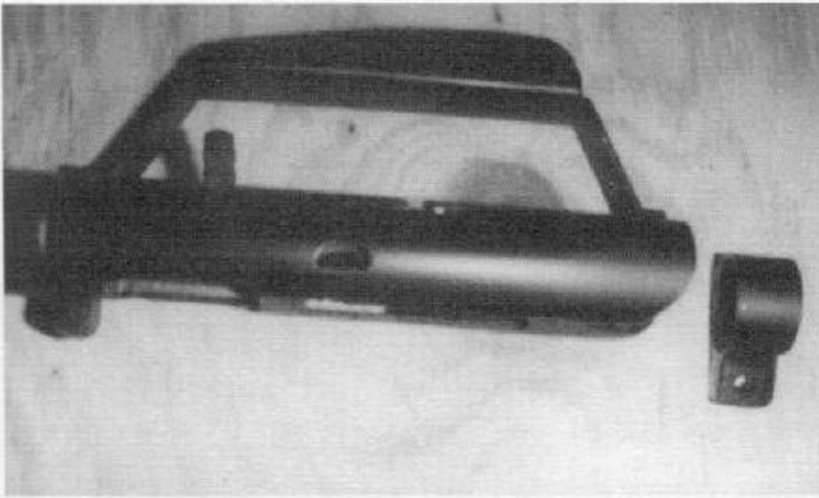
Cut near center to clear bolt release.
