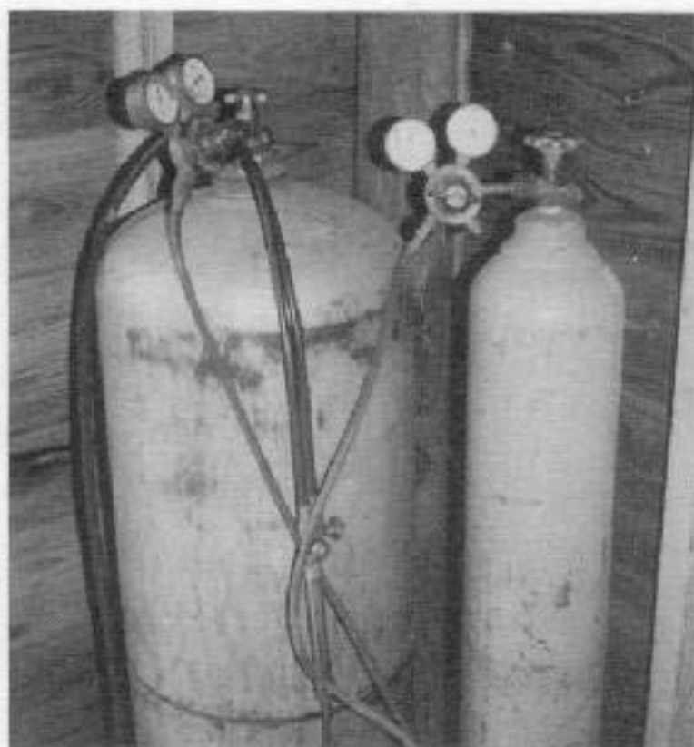
This gas welding set is used for silver-soldering, heat-treating, and coloring operations.
