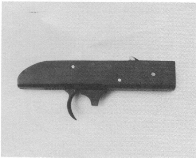
Above: Removable trigger assembly of the MP83A1.
