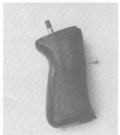
Grip can be shaped almost to final contour using disc sander.
