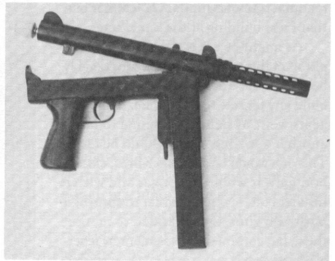
Below: The upper receiver tips up to allow bolt and trigger assembly removal.
