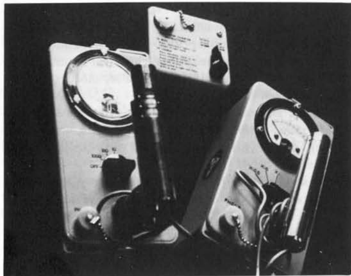
Individual dosimeters (top) are worn on the belt and are essential for counting the radioactivity each member of a group is exposed to. Survey meters (bottom) count the radioactivity in an area. Note the dosimeter charger pictured between the two survey meters.
