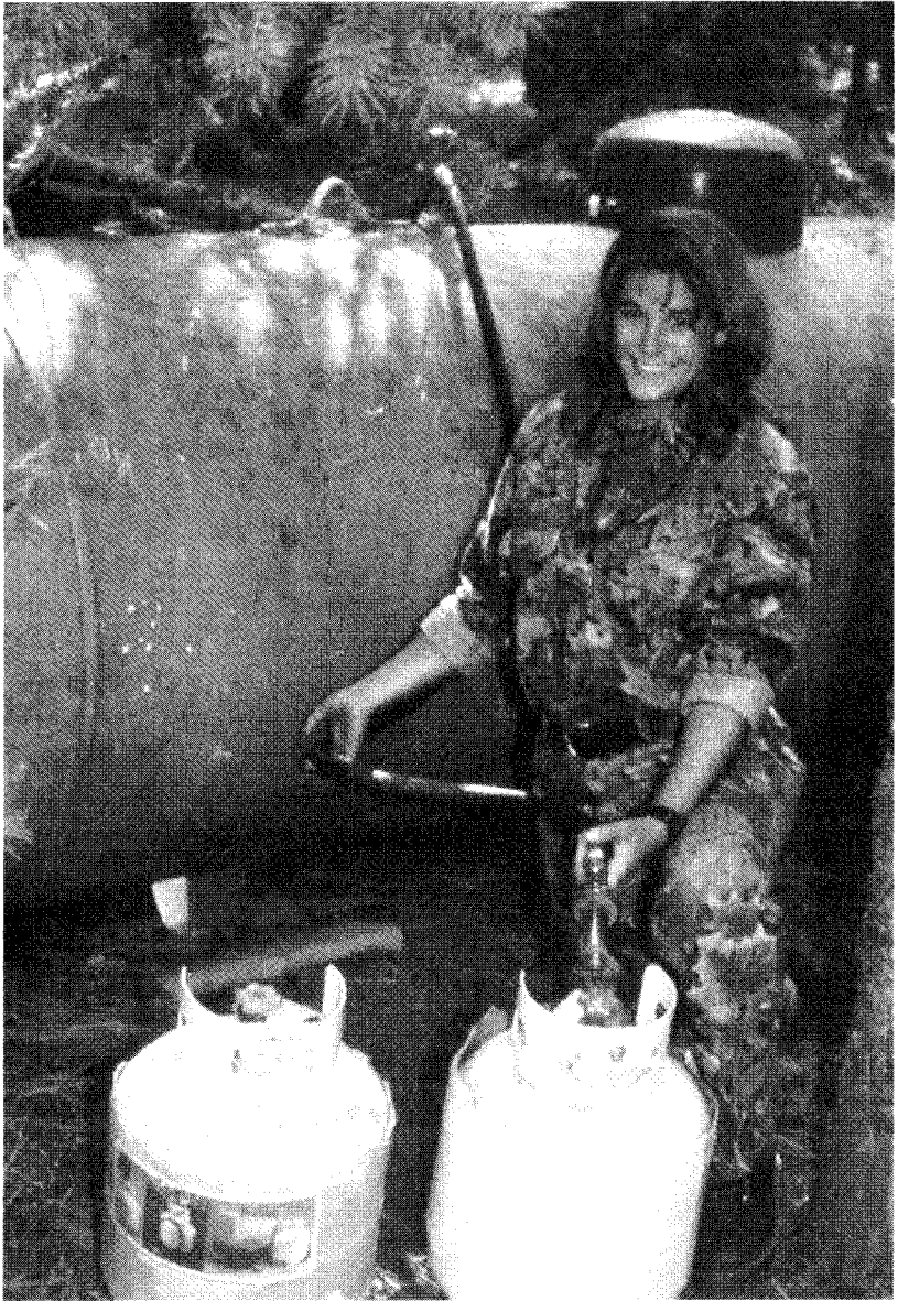
Small 5-gallon LP gas tanks can be filled from a large nurse tank if proper equipment is installed before the main tank is first filled.
