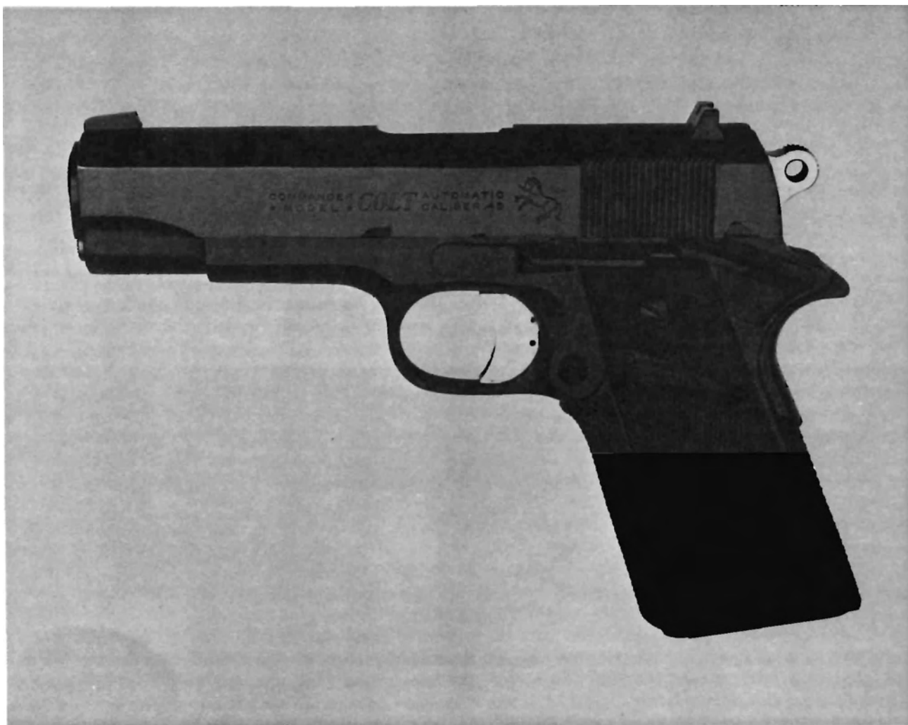
The Colt Commander .45 autopistol, one of the acceptable variants on the basic Colt design. This one has been customized for reliable operation in combat. Note the Pachmayr grips, the flat mainspring housing, the oversized slide release and safety levers, the King-Tappan fixed combat sights, and the long National Match trigger. Internal modifications (ramping, throating, and trigger job) were also performed. (Customizing by B&B Sales, North Hollywood, California.)
