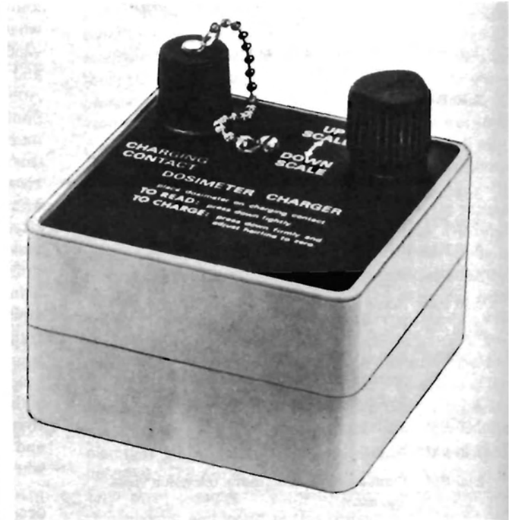
Individual radiation dosimeter and charger. This pen-like device gives a direct reading of personal radiation exposure. (Photograph courtesy of Nuclear Associates, Inc., 100 Voice Road, Carle Place, New York 11514.)
