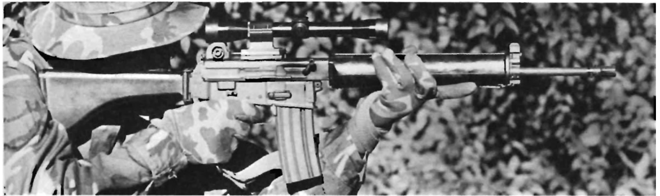
The Armalite AR-180 light assault rifle. Note the telescopic sights and the thirty-round magazine.
