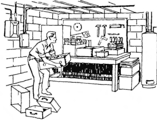
FIGURE 25: Two Expedient Basement Shelters. Shelters should be located in a corner of the basement beneath a sturdy workbench or table. Overhead mass is created by piling heavy objects in the room
