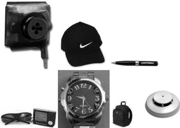
Figure 7-11 All of these devices capture audio and color video from a hidden camera except for the pen, which is an audio recorder.
