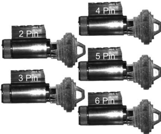
Figure 7-5 These see-through locks allow you to see how you are doing.
