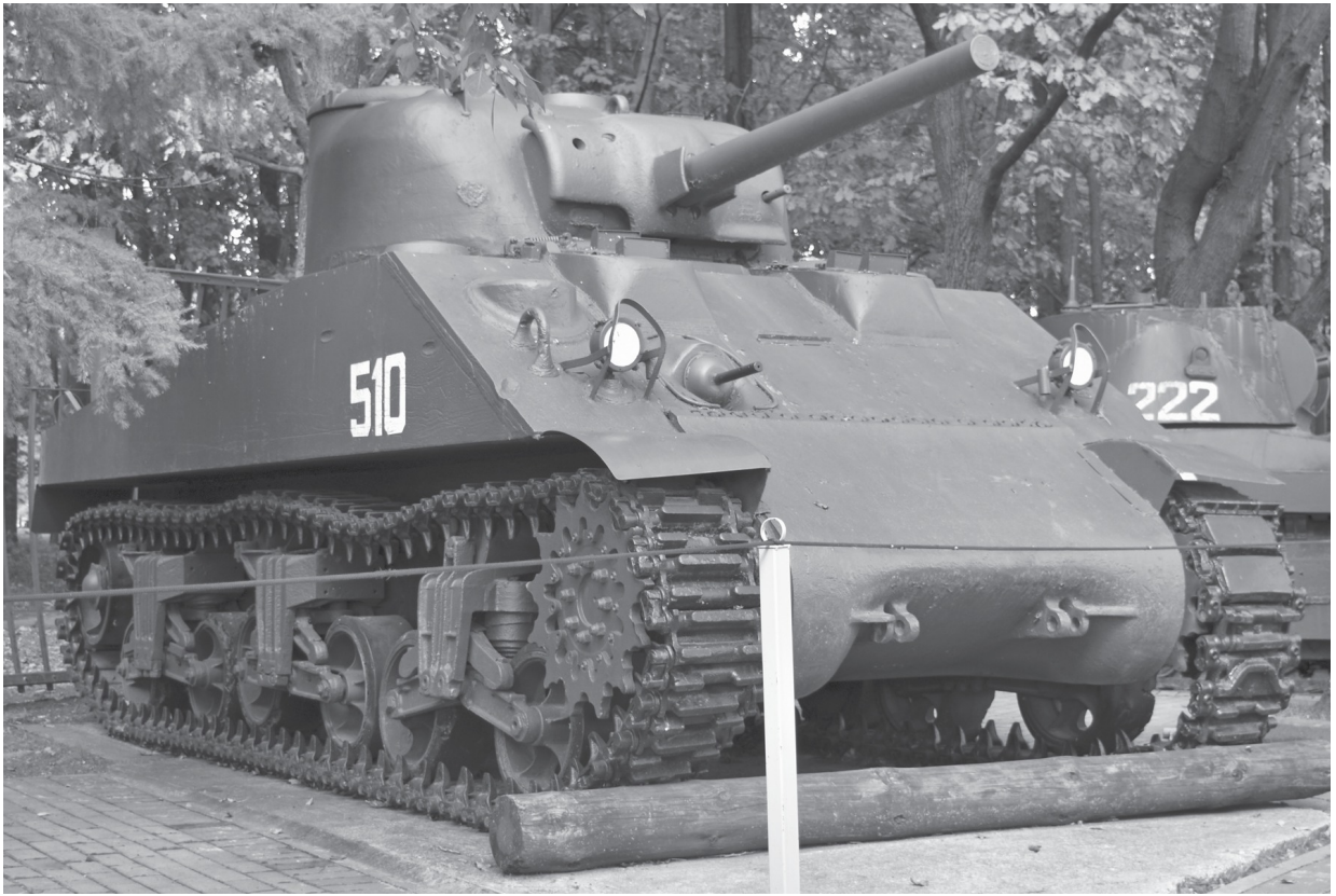
A diesel-powered American Sherman M4A2 tank, fitted with a 75 mm M3 L/40 gun, built exclusively for the Red Army. This one was restored by the Russian government in the 1990s. (Alan Wilson of Hawkeye UK.)
