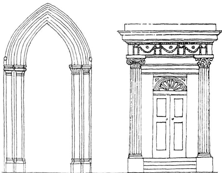
ON LEFT: A Gothic arch in which two different types of capital are satisfactorily combined. ON RIGHT: A 'classical' porch in which the introduction of dissimilar capitals introduces a jarring note.
