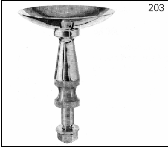
Left: Prop for the skull for a cubic craniophor. Weight: 0.300 kg. Right: Sighting device or cubic craniophor. (Schlaginhausen)
