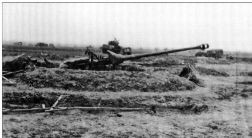
A number of these modified PaK 43/3 88mm guns were knocked out by the new Pershing tanks of the 9th Armored Division on the approaches to the Rhine. These weapons were intended for the Jagdpanther tank destroyer, but instead were adapted to a pedestal mount for use as an improvised anti-tank gun for Rhine defense. (NARA)
