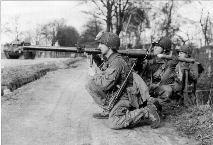
Among the new weapons first deployed during the Rhine fighting was the M18 recoilless rifle, here seen in action with paratroopers of XVIII Airborne Corps near Münster in late March 1945. Unlike the bazooka anti-tank rocket launcher, the recoilless rifle was designed to fire high-explosive rounds to provide lightweight fire support. (NARA)
