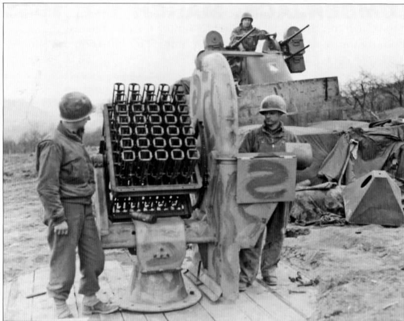
Among the weapons defending the bridge was the secret Flakwerfer 44 Föhngeräte of the 900th Flak Training and Test Battalion stationed on both sides of the river. This example was captured in Erpel and behind it is a US Army M16 anti-aircraft half-track of the 634th AAA Battalion (Automatic Weapon) guarding the bridge area. (NARA)
