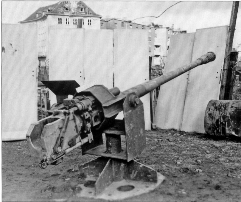
To help stiffen the Rhine defenses, armored vehicles' weapons awaiting delivery at local plants were hastily fitted to improvised pedestal mounts to create impromptu anti-tank guns. This is a 50mm KwK 39 gun of the type fitted to the SdKfz 234/2 armored car. (NARA)
