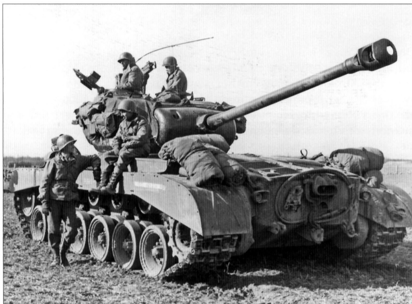
The attack on the Ludendorff Bridge was supported by a platoon of the new T26E3 Pershing tanks led by Lt. Grimball of the 14th Tank Battalion. This is one of the platoon's tanks seen on March 1 with its turret traversed to the rear in travel mode. (NARA)
