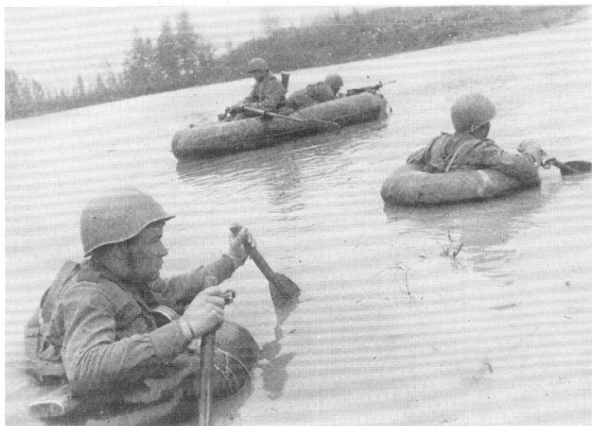
The Red Army had specialised river-crossing equipment for rifle division reconnaissance companies. These included the four-man LMN rubber raft and the MPK and PK rubber 'swimming suit'. The latter, seen in the foreground, included rubber trousers, to permit river crossing in cold temperatures, and paddles. (Sovfoto)
