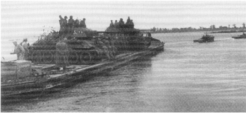
A river barge brings two Soviet T-34 Model 1943 tanks over the Vistula to reinforce the Sandomierz bridgehead. The barge is being towed by two Soviet BMK-70 motor boats, a standard Soviet engineer craft used for river-crossing operations. (Sovfoto)
