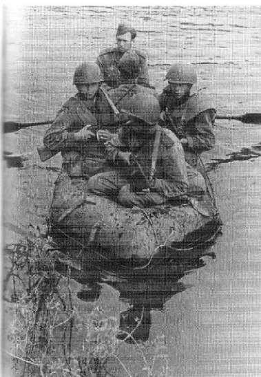
The initial bridgeheads over the San and Vistula rivers were gained by infantry units using rubber inflatable rafts. This example is called an LMN (small rubber boat), and was designed to accommodate five troops. (Sovfoto)
