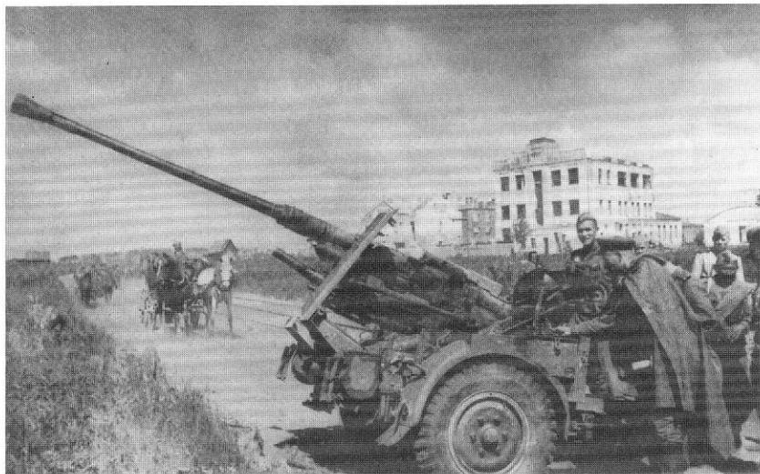
Red Army troops look over German war booty after the capture of Vitebsk. This is a 37mm Flak 36 anti-aircraft gun on a Sonderanhänger 52 carriage. (Sovfoto)
