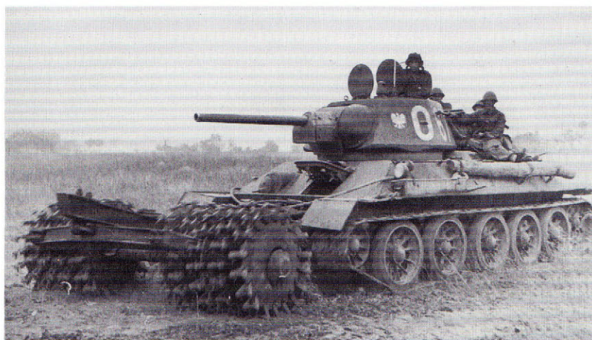
The fighting along the Moscow-Minsk highway near Orsha saw the first substantial commitment of Soviet armoured engineer equipment like the PT-34 mine-rolling tank. The German defensive belt on the main approach to Minsk forced the Soviet 11th Guards Tank Army to precede their infantry attacks with special armoured assault groups. This photo was taken after Operation Bagration, and shows a Polish PT-34. (Janusz Magnuski)
