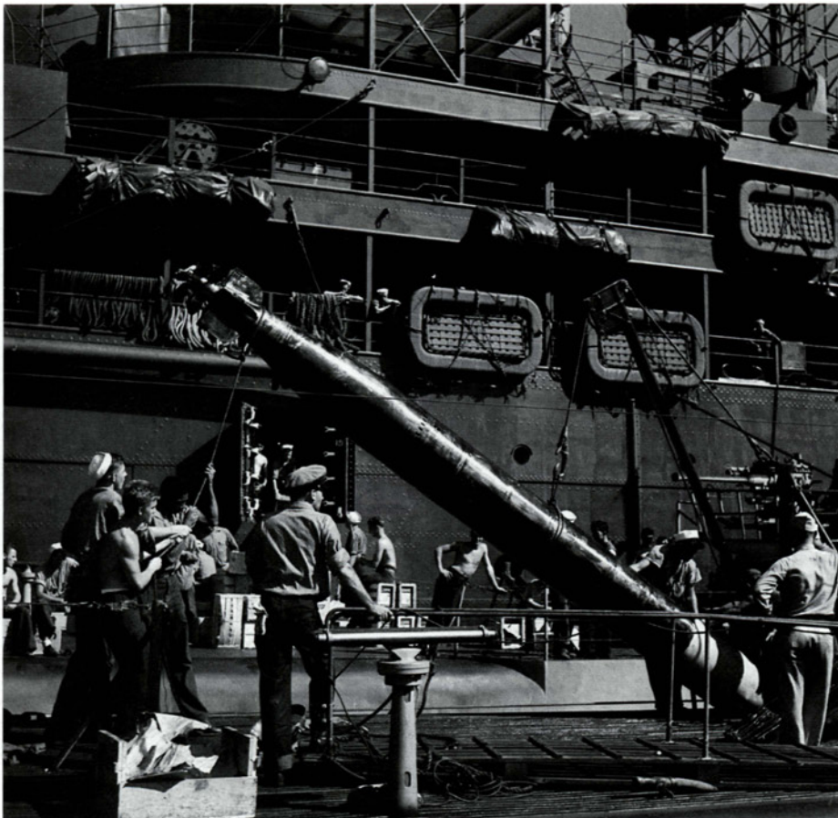
Alongside a fleet tender a submarine crew tackles the ticklish yet repetitive task of striking down the torpedo outfit. For a considerable period American torpedoes were notoriously unreliable. The T-shaped object in the foreground is a trainable Sonar hydrophone.
