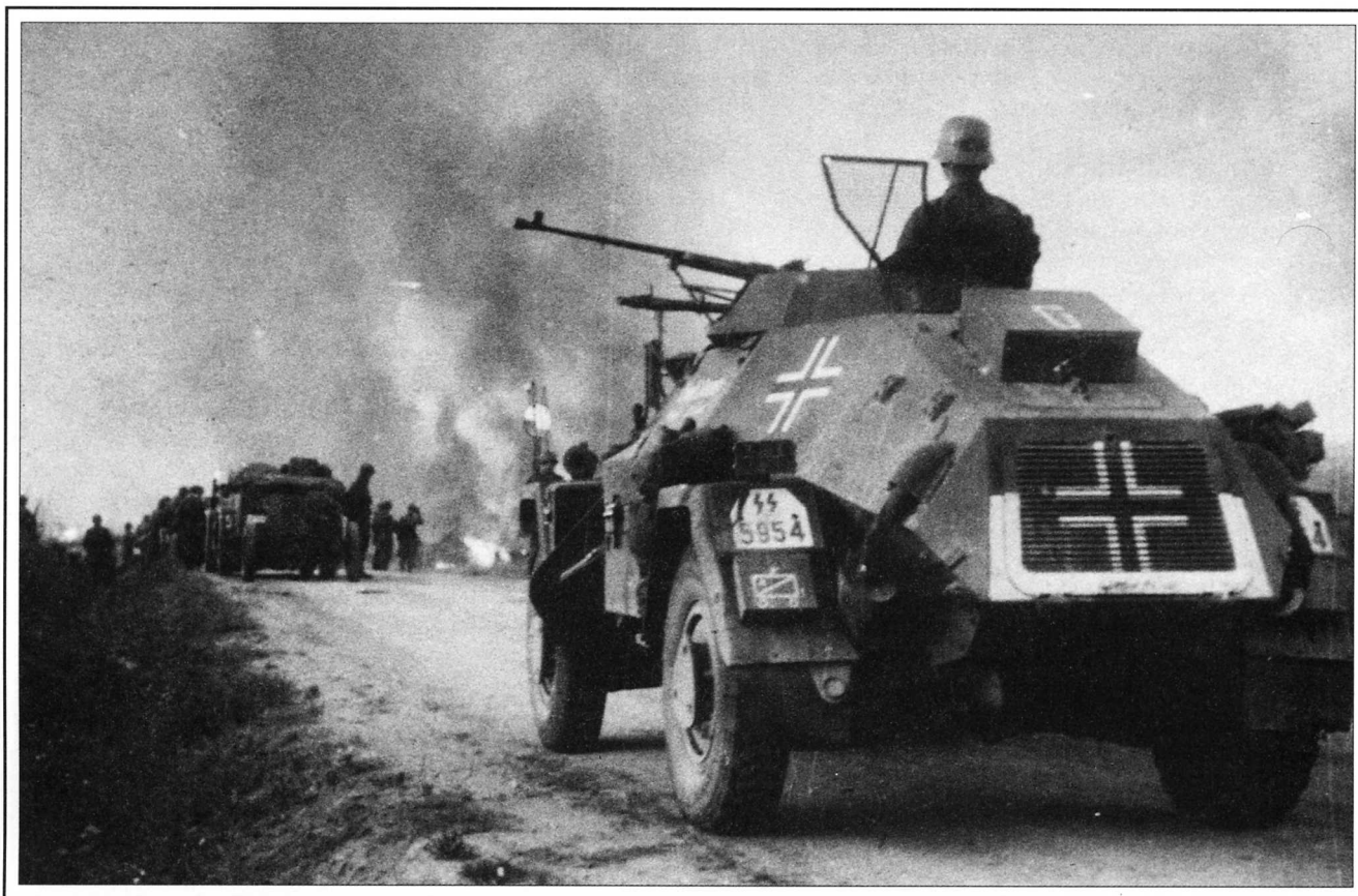
ABOVE: A Das Reich Division SdKfz 222 light armored car in Russia in the summer of 1941.
