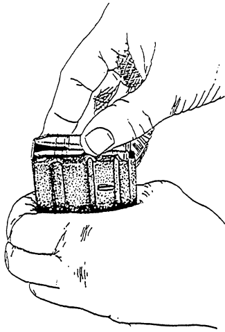
Figure 3-21.—Loading cartridges into the magazine, 20 rounds capacity.
