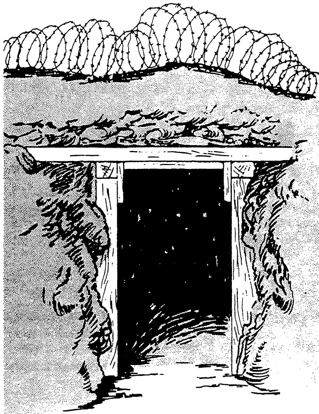
Figure 8-2.—Protective wire on top of overhead cover.
