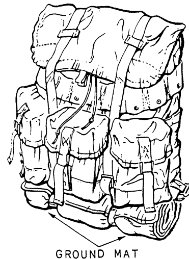
Figure 2-16.—Ground mat attached to medium pack.
