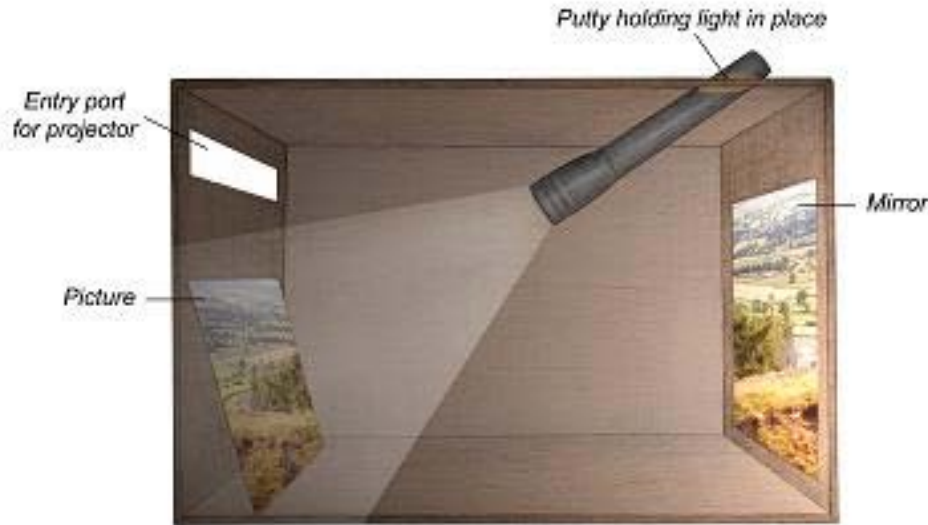
Fig. 26. Picture box setup with mirror
