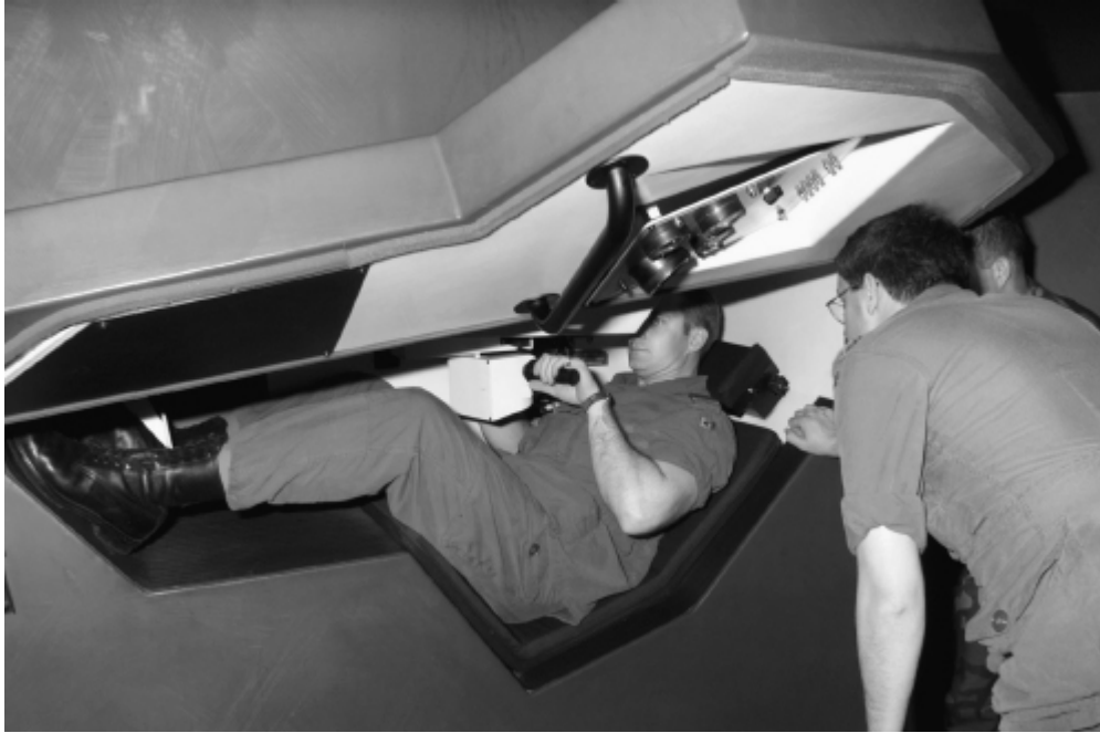
Students train in an M1 Abrams tank SIMNET simulator, the brainchild of DARPA's Jack Thorpe. (U.S. Department of Defense)
