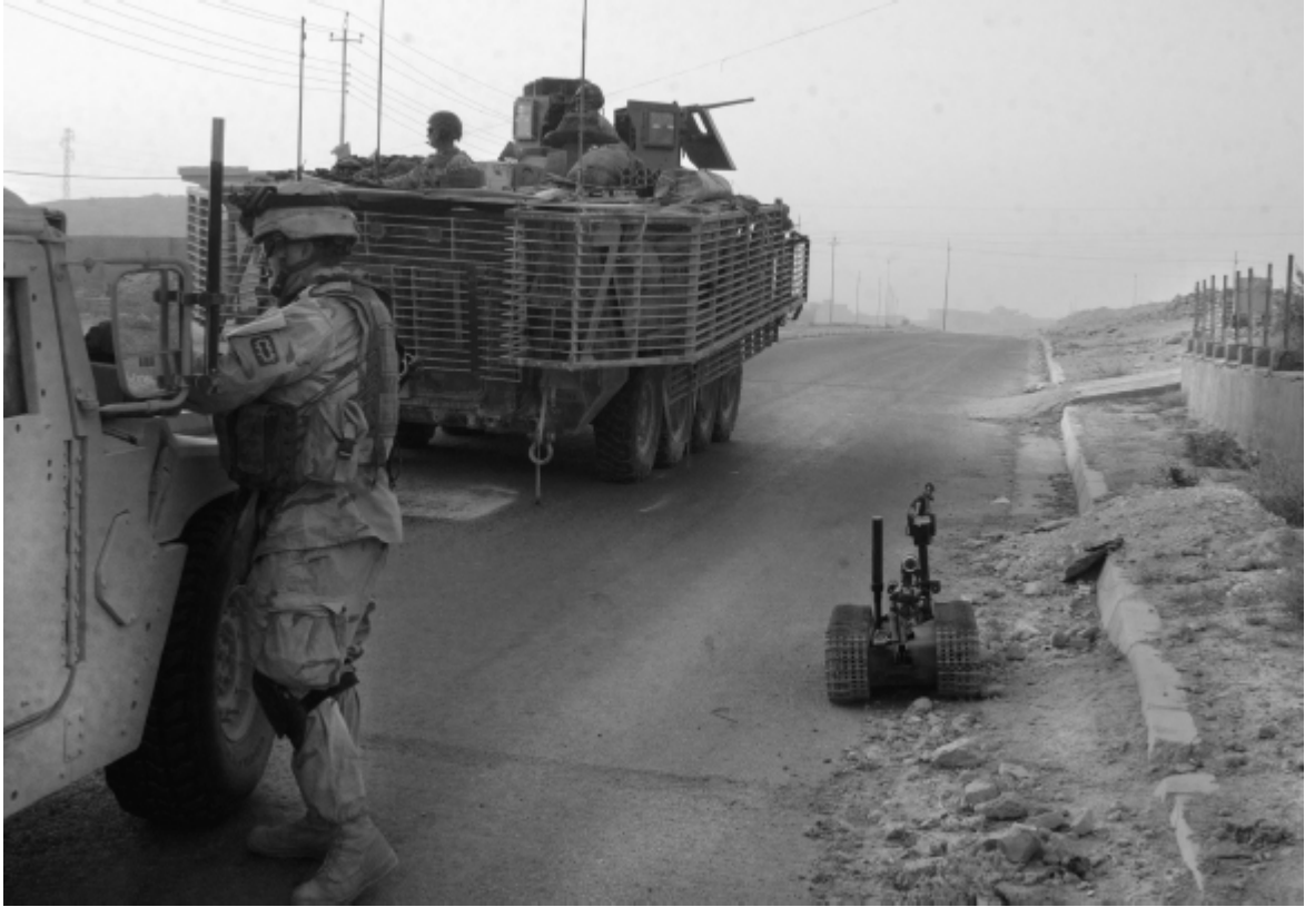
DARPA's Talon robot approaches a deadly improvised explosive device (IED) in Rajah, Iraq. (U.S. Army, photo by Specialist Jeffrey Sandstrum)
