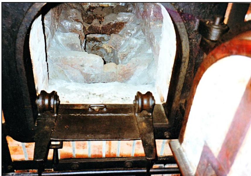
Document 40: Crematorium of Buchenwald. Topf triple-muffle coke-fired furnace. Central muffle. Roller device for coffin-introduction cart (Sargeinführungswagen) in position for operation. © Carlo Mattogno.
