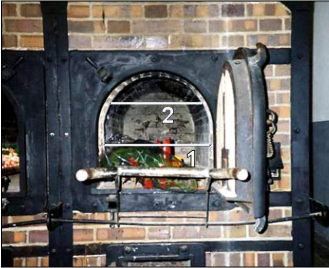
Document 46: Crematorium of Mauthausen. Topf coke-fired double-muffle furnace Auschwitz type. (Cf. Document 43). The two horizontal lines represent the height of two superimposed normal corpses on the muffle grid.
