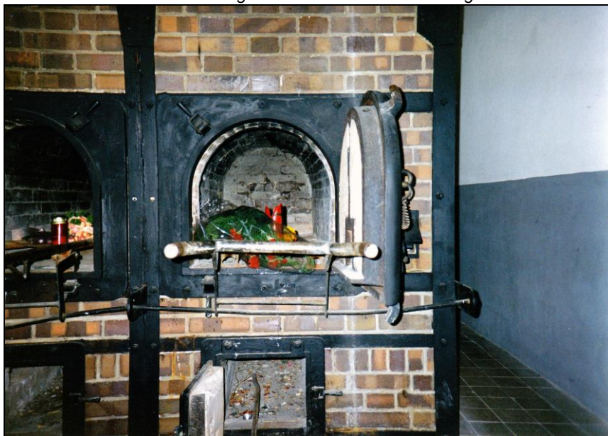
Document 43: Crematorium of Mauthausen. Top coke-fired double-muffle furnace, Auschwitz Type. Loading system of furnace: fixation shaft, mobile roller system, and corpse stretcher. Front view. © Carlo Mattogno.
