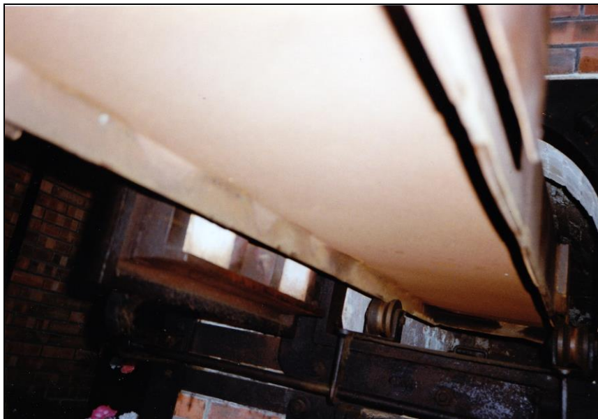
Document 42: Crematorium of Buchenwald. Top triple-muffle coke-fired furnace. Central muffle. Corpse-introduction cart. Lower side. Rims of the stretcher running on the rollers. © Carlo Mattogno.
