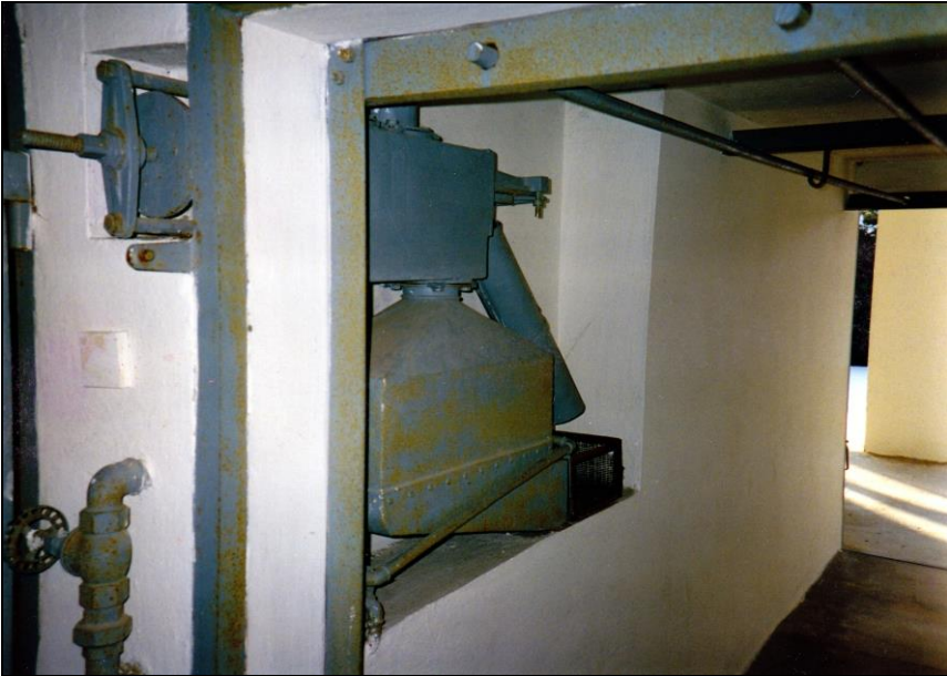
Document 13: Photograph of circulation device of a disinfestation chamber using HCN gas (Zyklon B) with the Degesch-Kreislauf system at the Dachau camp. © Carlo Mattogno 1990.
