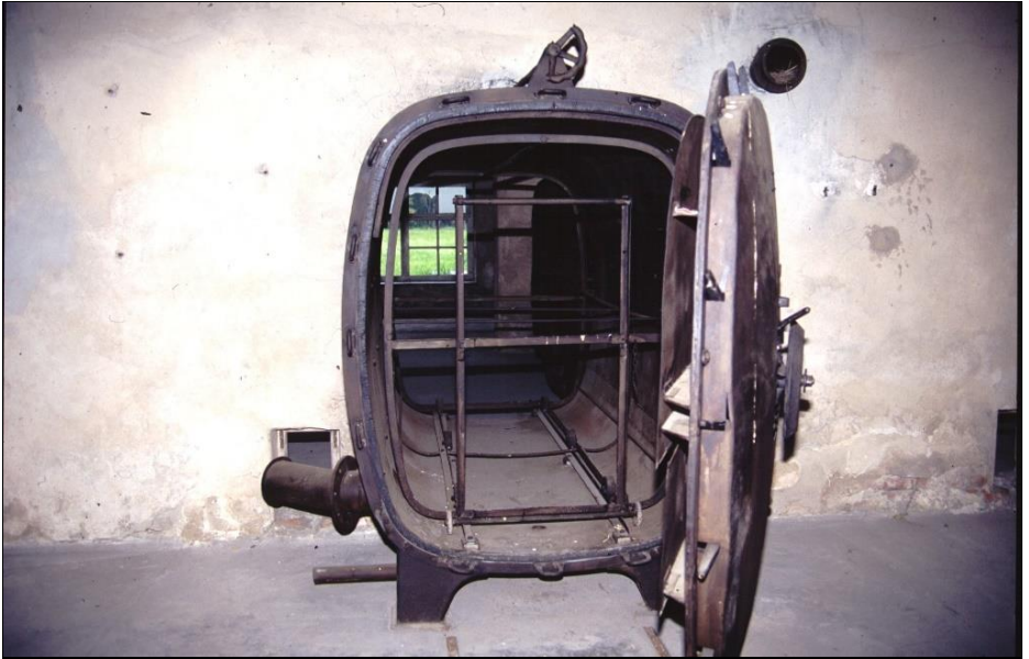
Figure 36: Autoclave for steam disinfection inside the so-called “Zentralsauna” in Auschwitz-Birkenau (Leuchter et al. 2017, p. 221).
